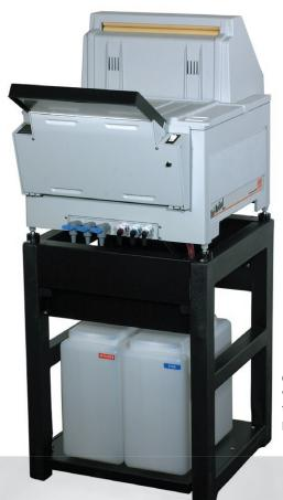
Comes ready to set up, complete with a sturdy base stand, 7 gallon tanks, connector hoses and starter parts kit all included.
